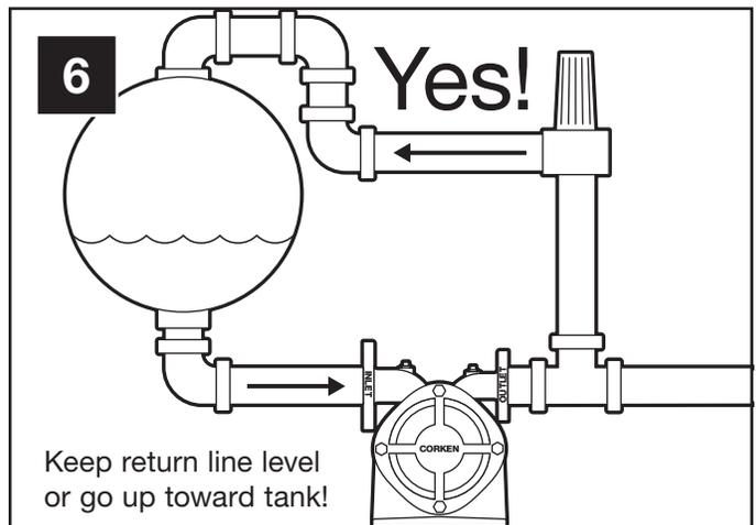
Low spots in bypass line can collect liquid which prevents normal vapor passage for priming purposes just like the P trap in the drain of a kitchen sink. This is not a problem for bypass lines where vapor elimination is not required.
