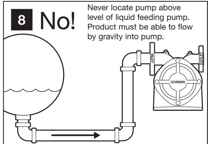
Since liquefied gases boil when drawn into a pump by its own suction, the pump must be fed by gravity flow to give stable, trouble-free operation.
