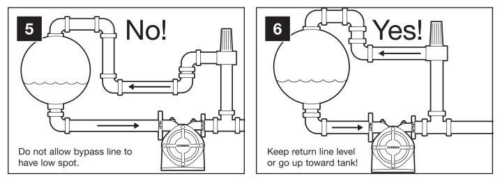
Low spots in bypass line can collect liquid which prevents normal vapor passage for priming purposes just like the P trap in the drain of a kitchen sink. This is not a problem for bypass lines where vapor elimination is not required.
