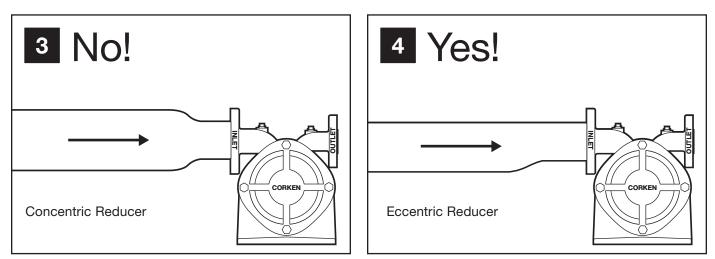
An eccentric reducer should always be used when reducing into any pump inlet where vapor might be encountered in the pumpage. The flat upper portion of the reducer prevents an accumulation of vapor that could interfere with pumping action.
