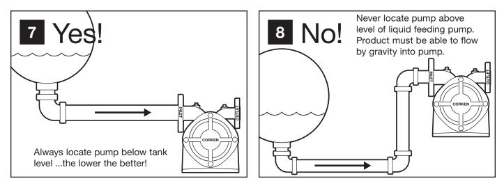
Since liquefied gases boil when drawn into a pump by its own suction, the pump must be fed by gravity flow to give stable, trouble-free operation.
