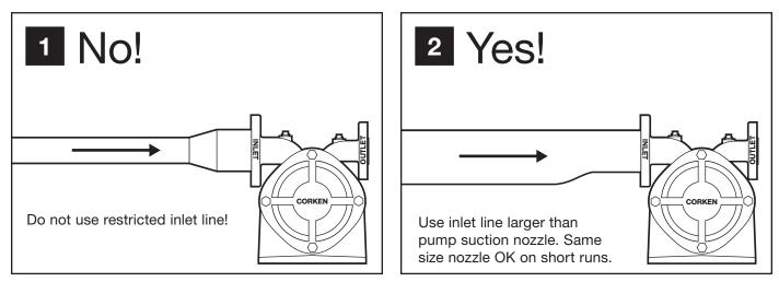
Pressure drop caused by restriction in suction line will cause vaporization and cavitation.
